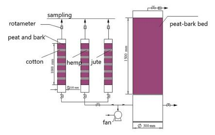
Figure 2. Schematic diagram of the test rig consisting of biological beds filled with a mixture of peat and bark, jute, hemp and cotton
