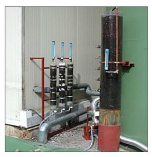
**Figure 1.** Test rig for deodorisation of industrial gases using peat-bark filled biofilters and biofilters with plant fibre layers
